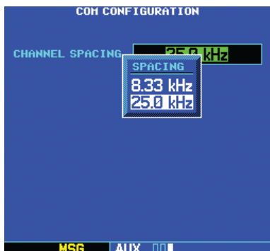
Figure 10-44 Channel Spacing Window
