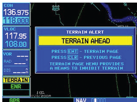
Figure 12-4 TERRAIN Caution Pop-up (Flashing)
